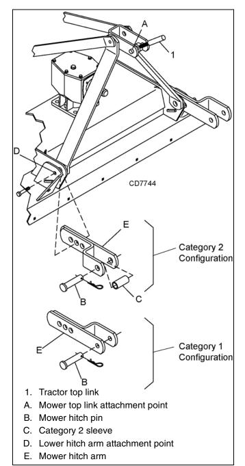
Figure 29. Hitch Arm Installation
